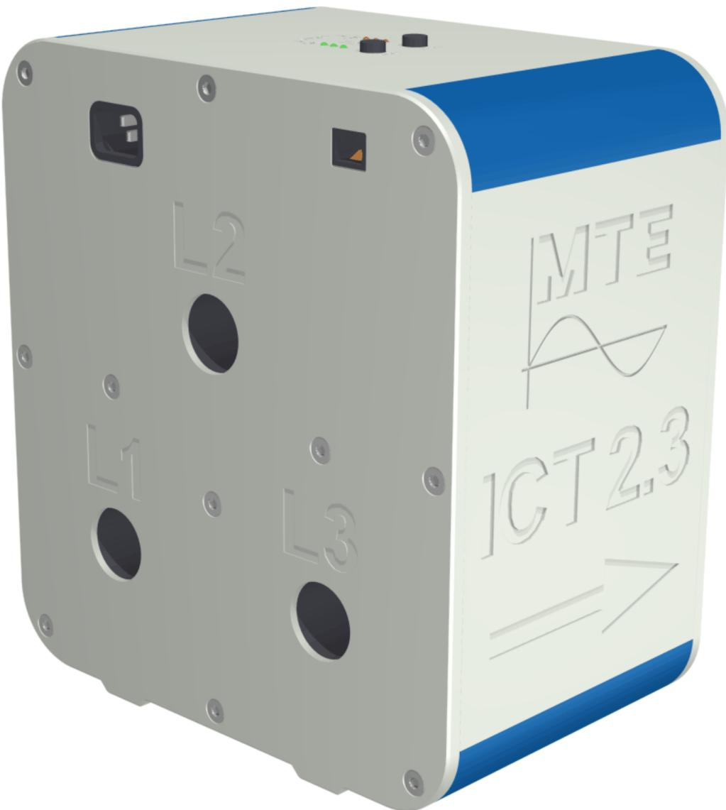
The ICT 2.3 three-phase Isolation Current Transformer is used on multi position test benches for testing three-phase meters with closed links between the current and voltage measuring circuits (C-P links). Meters of this type are produced and used with increasing frequency.
